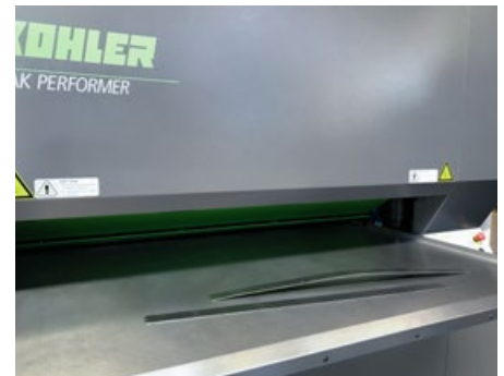
Before and after: The parts are even and low stress (front) after leveling and can therefore be processed faster and better. The results are higher quality products. The unlevelled sheet can be seen at the rear for comparison.
