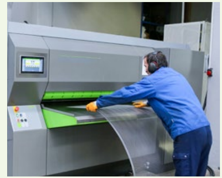
Leveling perforated sheets on a Peak Performer 30P.1250 with roller bending Image: Özselin Perforated Sheet Ltd. Co.
