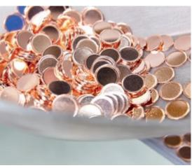
Top image: Coin blanks and leftover stamping scrap. Freiberger EuroMetall GmbH manufactures a variety of sizes of coin blanks. The blanks are manufactured in huge batches of millions of pieces from a large strip width of material and with constant precision.
