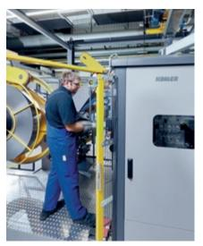
The strip is inserted into the strip leveling machine manually
