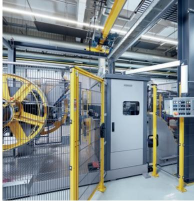
Freiberger EuroMetall uses stamping and edge rimming to produce their coin blanks. The preliminary work is performed by a KOHLER strip feeding line comprising (from left to right) a double decoiler, strip leveling machine and strip transfer to high speed punching machine
