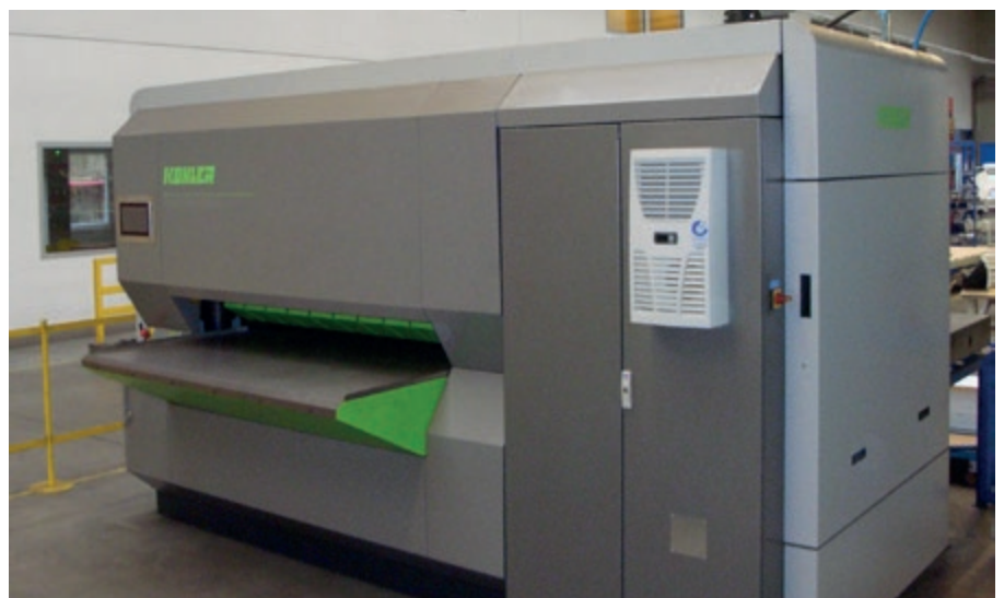
The servo electronic Peak Performer 50P part leveling machine impresses with innovative technical features such as the electromechanical leveling gap control and the advanced cleaning system.
