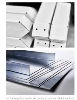
which are fully perforated, cut to length and either a) painted or b) galvanized, are given their profile contour in a subsequent bending process, which is dependent on the application
