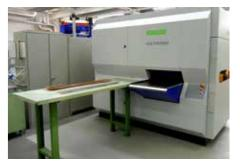
The compact and neatly enclosed Peak Performer 50P.600 part levelling machine, viewed from the outlet side. The levelled precious metal strips are deposited on the table.
