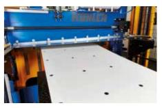
The cut-to-length shear cuts the strip to the precise length of the later edge profile
