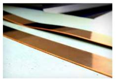
The levelling result achieved by the Peak Performer 50P.600 is clear; at the top you see the (gold) strip prior to levelling, and below is the levelled, even, absolutely flat strip.
