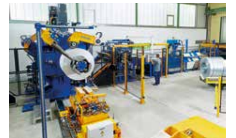
— An overview of the entire production line (from left), with coil preparation, coil loading car, double-sided decoiler, levelling machine, loop pit, hole punch, and cut-to-length line.
