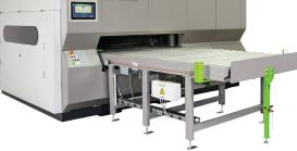
KOHLER Peak Performer, a hydraulic-free part levelling machine
