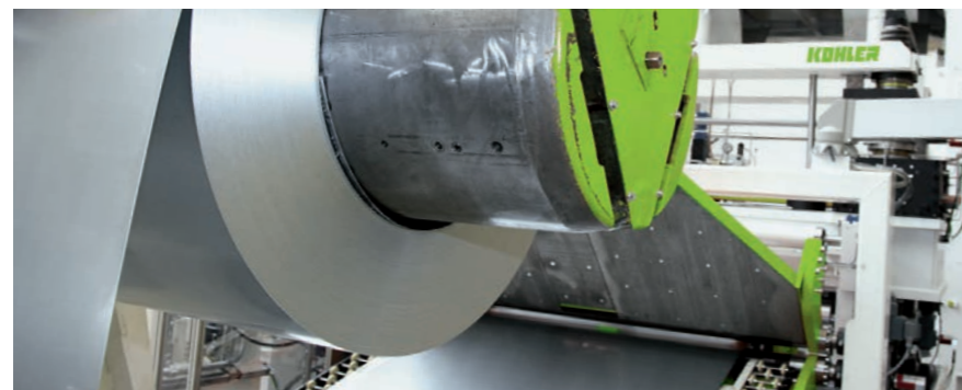
— Coiler with leading-in device
