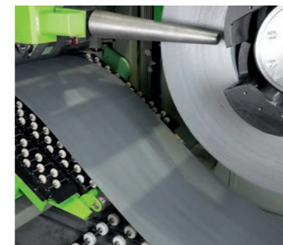
— Strip threaded into levelling machine
