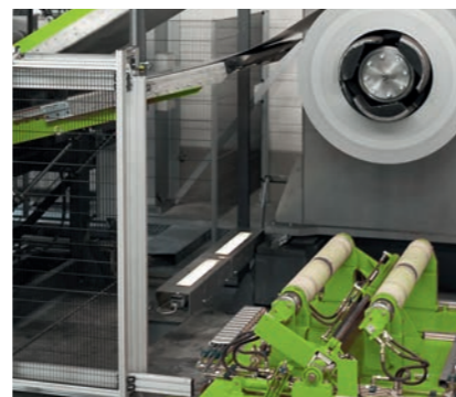
— Coil loading car in front of coiler
