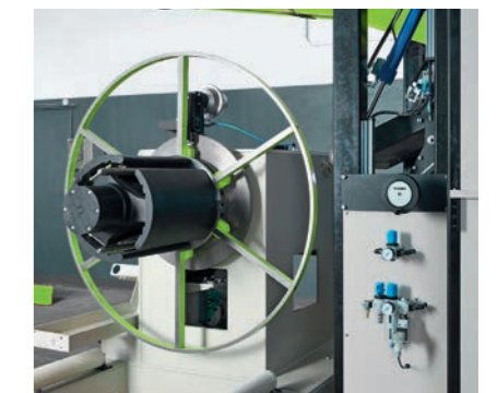
— single-sided coiler with transversing device
