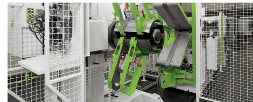
— Decoiling side of a double-sided coiler
