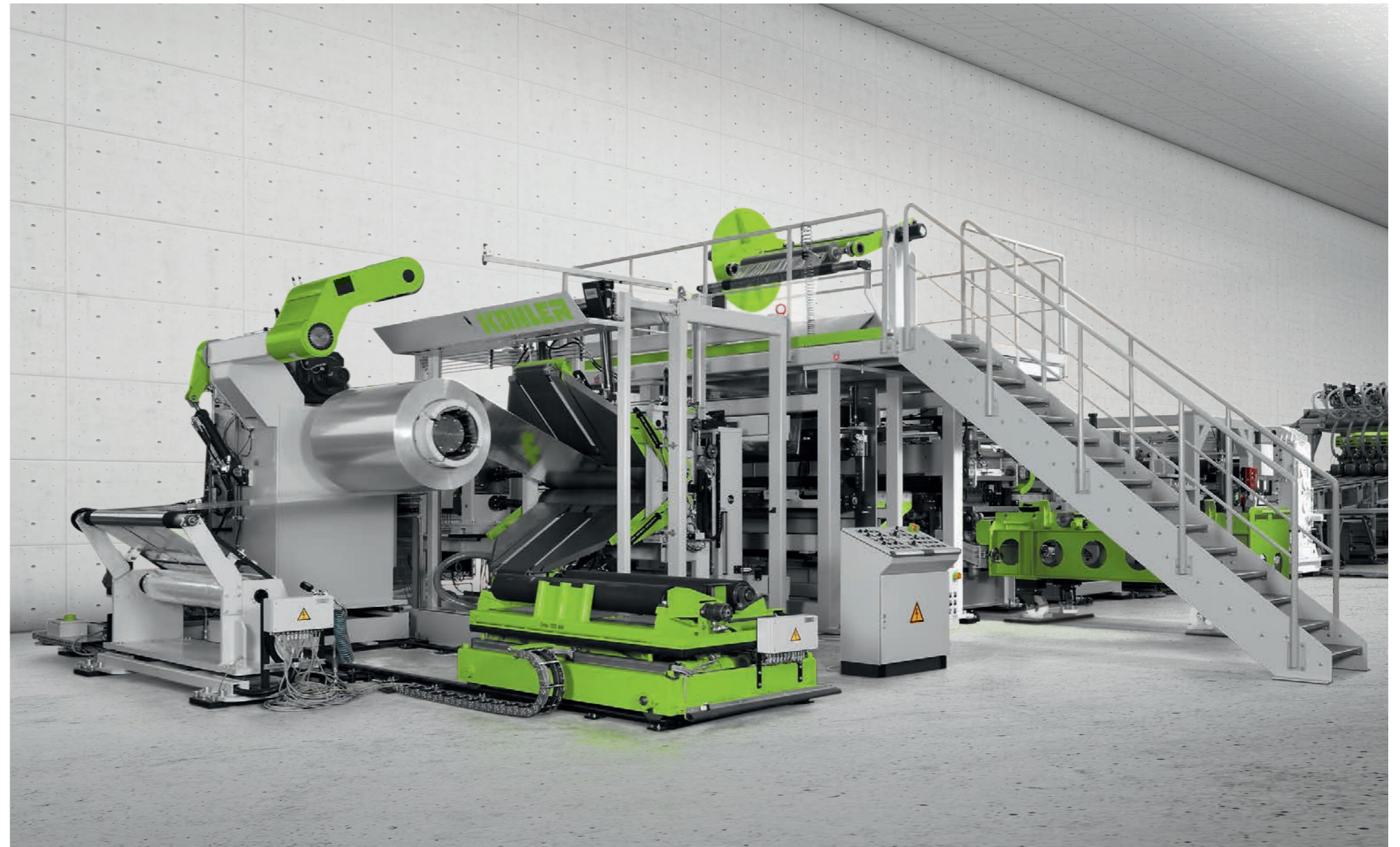
— Cut-to-length line with vacuum stacker for highly surface-sensitive blanks
