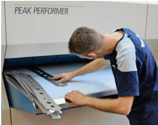
The machine is safe and shuts down when the operator gets too close to the levelling rollers.
