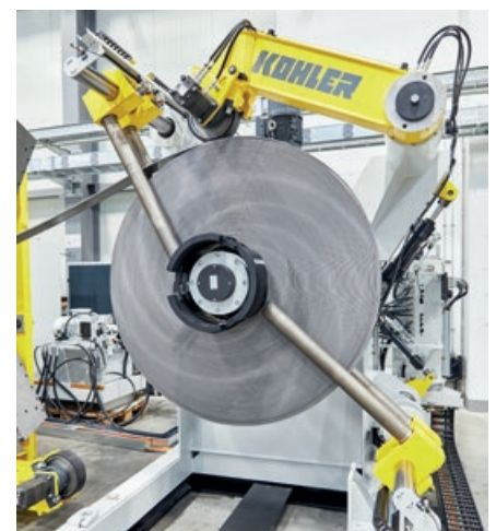
Coil loading chair and decoiler can be delivered with a capacity of up to 35 tons.
