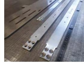
The longitudinal and transverse struts as well as the base panels of the frame are leveled before assembly, in order to satisfy the high requirements for levelness and precision, and to eliminate tension in the material. Photo: German institute for the research and development of sports equipment (FES)
