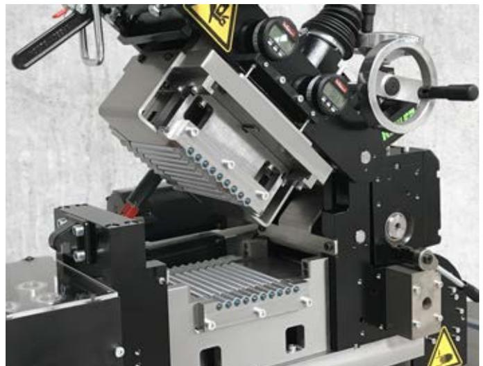
Easy accessibility allows for quick and straightforward cleaning of supporting rollers and leveling rollers.
