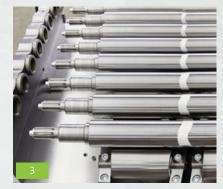
Patented reversible leveling rollers
